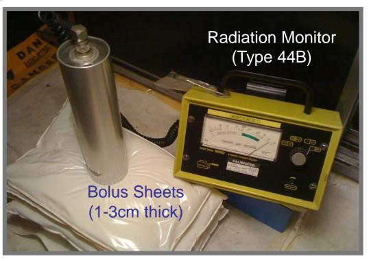
Measurements (cps) showed a seed could be located up to 15cm deep in a person with the radiation monitor away from the surface of the body
